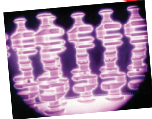
PRECISION MACHINE GROUND, HEAT-TREATED AND NITRIDED
