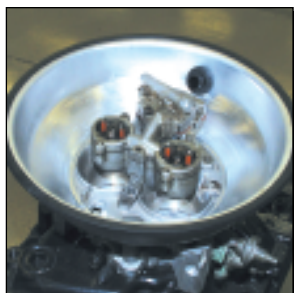
Stock throttle body and Power Charger
