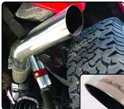
Diesel systems come with laser etched, polished 304 stainless steel tailpipe
