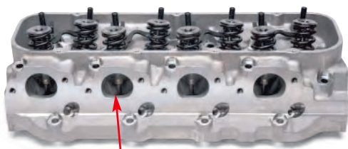
Exhaust ports are raised .630" over cast iron stock heads
