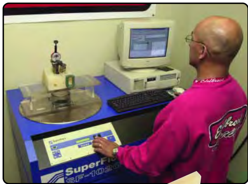
Edelbrock engineers test a cylinder head "flow box" on our SuperFlo SF-1020 flow bench
