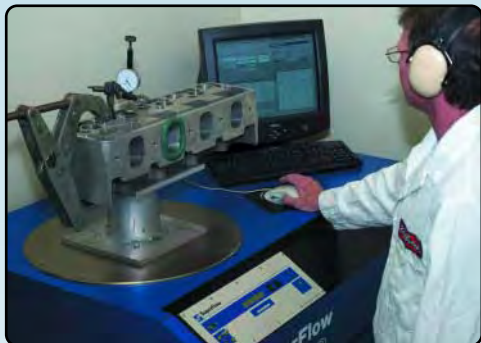
Traditional methods of cylinder head testing have been upgraded with computer monitoring for precise evaluation
