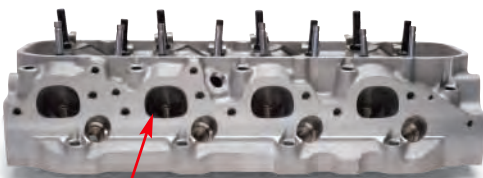
Casting "rolled over" 1.5° before machining for smaller combustion chambers and improved intake port alignment Victor Jr. CNC #60429
