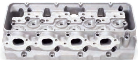
Hot Isostatic Pressing creates a super strong A-356 aluminum casting for superior durability and better machined finishes
