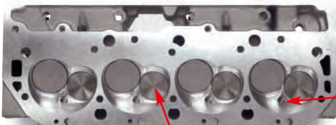
Edelbrock/Musi heads include large 2.30" intake and 1.90" exhaust valves
