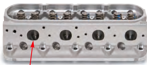
76cc exhausts flow 200 cfm at 0.550" valve lift
