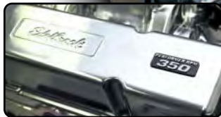
Performer RPM crate engines include Edelbrock aluminum valve covers with a custom badge
