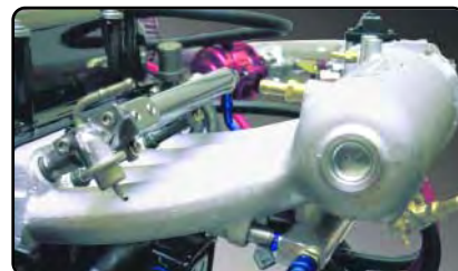
#4756 with Fuel Rail Upgrade Kit #4752 installed
