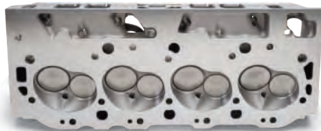
Performer RPM 454-R #60559 has 118cc combustion chambers with 2.19"/1.88" stainless steel, swirl-polished valves
