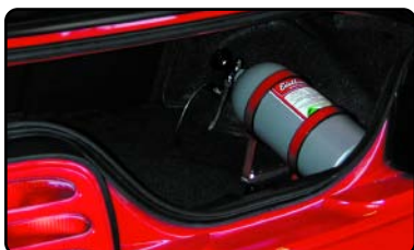
Edelbrock Nitrous Bottle installed in a 1994 Ford Mustang 5.0L
