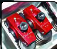
Includes red roller rockers made by Crane Cams
