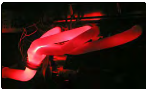
Edelbrock Ti-Tech coated headers look like new even after hours of brutal testing on our engine dyno
