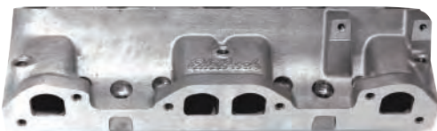
Performer RPM Pontiac Semi-Machined head #60509 is not drilled for the intake pushrods, allowing custom intake port widths using offset lifters or rockers
