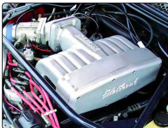
An Edelbrock Performer intake manifold #3821 tops off this 5.0L Mustang
