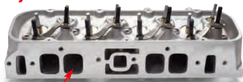
Partially CNC-ported, standard location 295cc oval intake ports Victor Jr. CNC #60429
