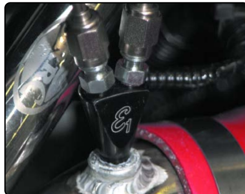
#72555 installed on cold air intake tube
