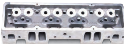
Victor 23° High-Port #77559 has .200" raised intake runners... same casting used for Victor CNC heads
