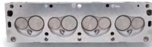
Performer RPM FE for 390-428 Cobra Jet #60069 has 72cc combustion chambers and 2.09"/1.66" valves for increased flow
