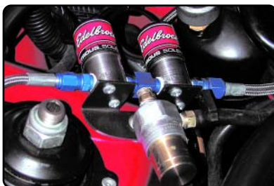
EFI Dry Nitrous Kit installed on a 1994 Ford Mustang 5.0L
