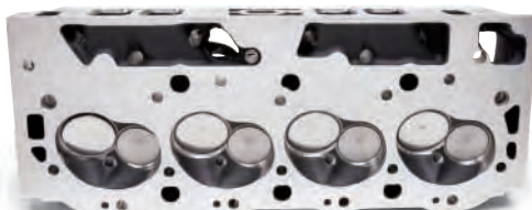
110cc combustion chambers are fitted with stainless steel 2.25" intake valves and 1.89" Inconel exhaust valves
