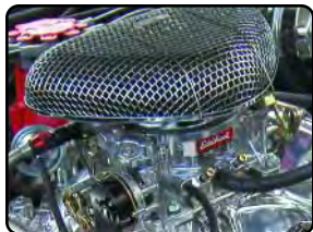
The Pro-Flo 1000 Series air cleaner looks great on this S/B Chevy with a polished Edelbrock manifold.
