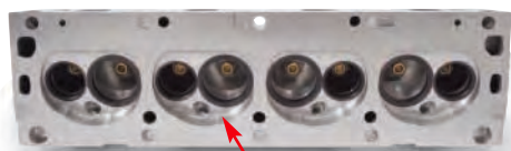
Performer RPM FE head #60087 has 76cc combustion chambers and accepts 2.09"/1.66" valves (427 low riser sizes)
