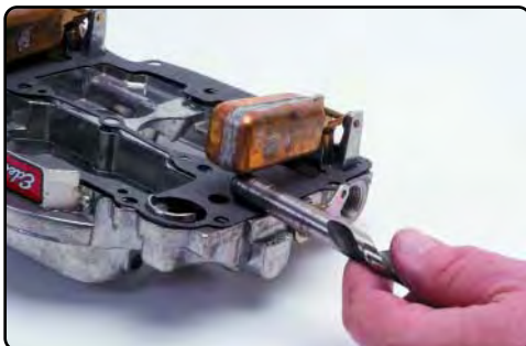
Checking float level with a 7/16" drill bit
