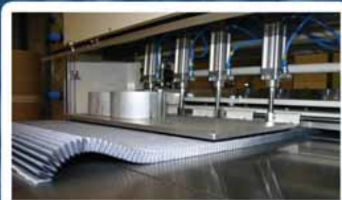
Perfect high flowing pleats come from a carefully designed pleating line and custom assembly jigs to hold the pleats in position during molding.
