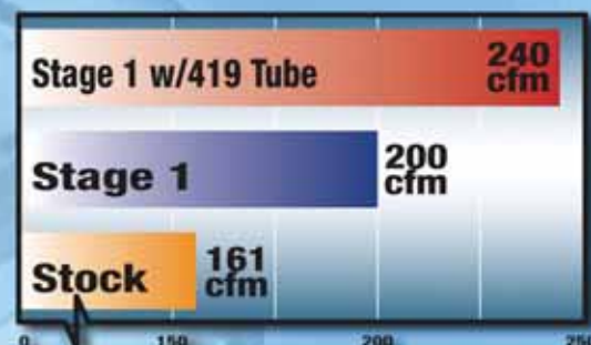
Airflow Comparison (CFM) @ 1.5" H2O Flow comparison based on '03 2500 California model Cummins.
