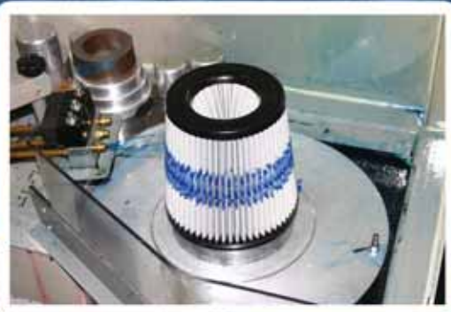
Perfect oil coverage comes from automated oilers.
