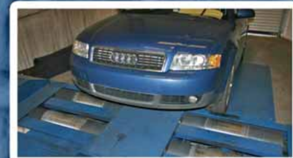
The prototype is installed and Dyno tested. Several revisions may be tested until the ultimate power gain is achieved.
