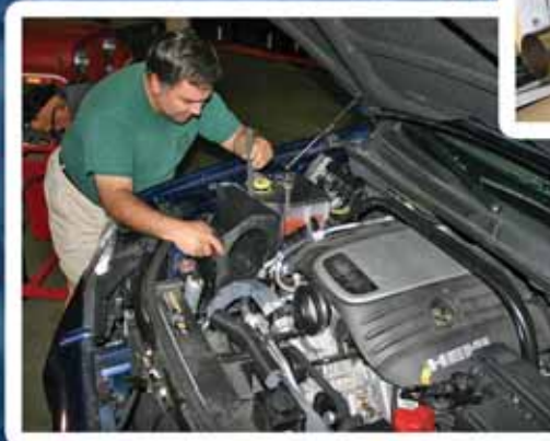
Dimensional mock-ups of the air box are welded and test fit until perfect.
