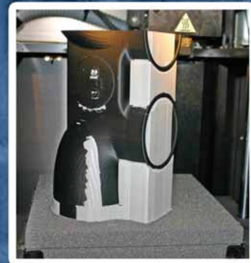
The three dimensional drawing is "printed" on a 3D printer, resulting in a prototype part that is fitted to the vehicle.
