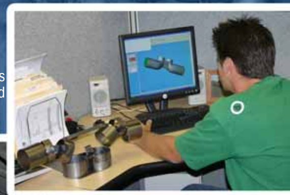
The mock-up digitization is rendered into a full scale three dimensional drawing.
