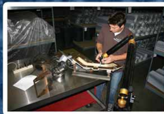
Mock-ups are digitized and imported into a CAD program.
