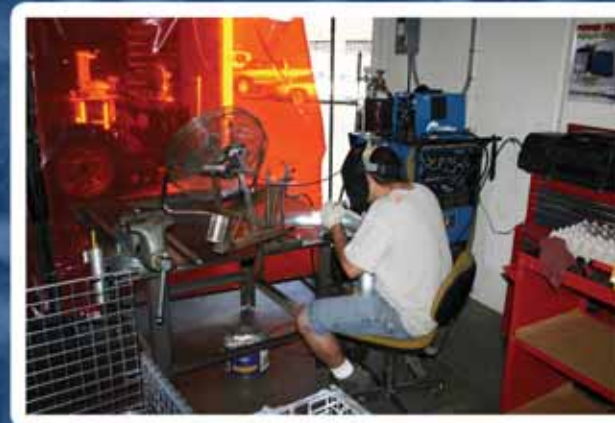
Dimensional mock-ups of the air box are welded and test fit until perfect.
