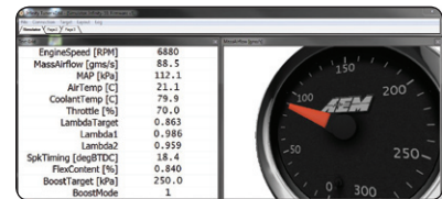
Infinity system models are purely airflow based, eliminating the need to reference lookup tables for injector pulsewidth.
