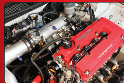
B-Series Coil On Plug Conversion kit installed on B18 engine.
