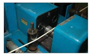
An optical laser measuring device keeps constant measurement on the completed wire as it comes to the end of the line. The machine operator must maintain the measurement within a specified amount and adjust as necessary.
