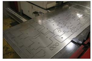
This turret punch press machine is where Moroso's precision manufacturing process begins. Small reference holes become precision cuts, and finally turn into an entire sheet of pre-cut aluminum components. Once a design program is entered into the machine's computerized interface, the exact tolerances of the original pan can be repeated continually.
