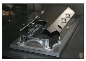
This photo shows the actual foundation after one of the billet end rails was welded in place. Moroso Oil Pans are truly precision-made products that cannot be mass produced with the same degree of accuracy and workmanship.
