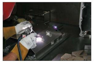
**Pro Eliminator Oil Pan (Part No. 20385)** uses several welded bungs for its various attaching points. It also features a billet rail for optimum sealing. The fixture is one-inch thick plate to absorb heat and ensure proper alignment, while preventing warpage.
