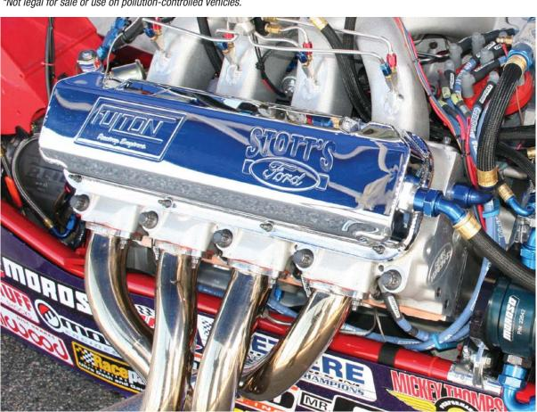
As demonstrated on the STOTT'S FORD Dragster, Moroso Fabricated Valve Covers can be etched, chromed, powder-coated or polished for a custom look.
