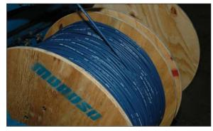
In the last step in the manufacturing process, completed wire is rolled onto wooden spools. Each spool holds 5,000-feet of wire awaiting the final steps to complete a length of spark plug wire.
