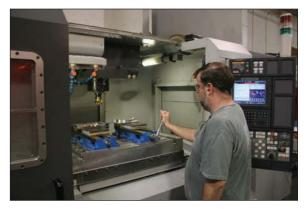
The billet aluminum end caps are precision milled on Moroso's bank of CNC machines.
