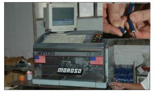
This automatic machine cuts the wire from the bulk spools to specified lengths and strips back the insulation on both ends prior to the terminal end crimping process.
