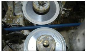
These print wheels are laser engraved with the Moroso and Ultra 40 Race Wire logos. At the end of the forming line, the wheels pick up ink and print on both sides of the wire.
