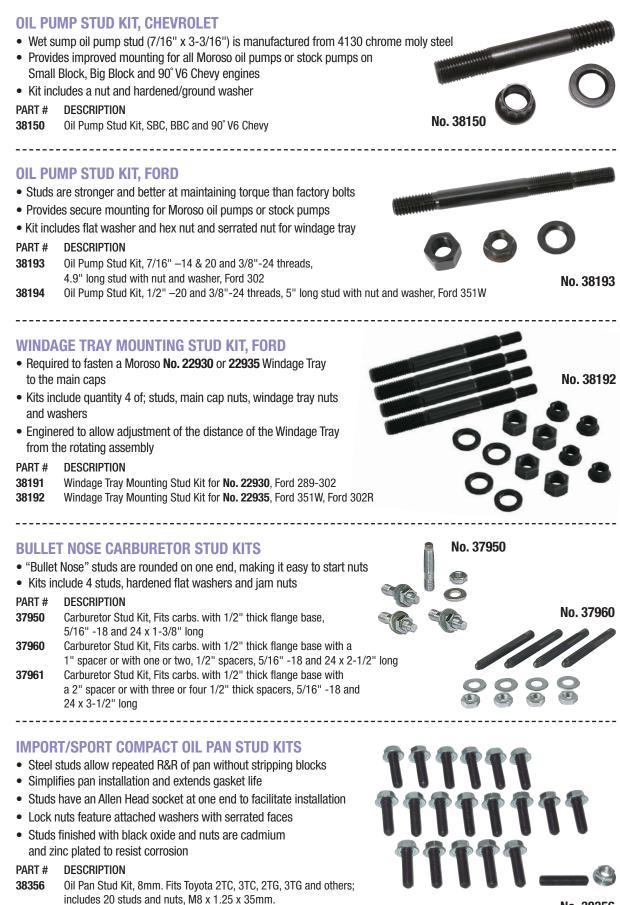
**38366** Oil Pan Stud Kit, 6mm. Fits Honda, Acura, Mazda Rotary, Dodge Neon, Toyota MR2 and others; includes 22 studs and nuts, M6 x 1.00 x 35mm.
