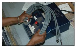
Before a plug boot is installed, each wire undergoes testing to ensure the quality of the crimp and the wire's conductivity. The plug boot is then installed, the wire is packaged and is ready for delivery.
