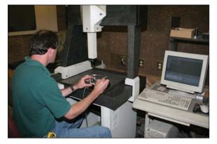
In Quality Control, end caps are computer checked for dimensional accuracy before transfer to manufacturing. A granite surface table works in unison with computerized digital probes in performing a battery of QC tests on a CMM machine, which is a staple in the aerospace industry.
