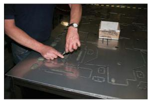
Similar to model car kits where parts are attached to "trees" for removal, each component of a fabricated oil pan must be manually detached from its parent sheet of aluminum. The individual pieces are then moved to the manufacturing department for assembly.
