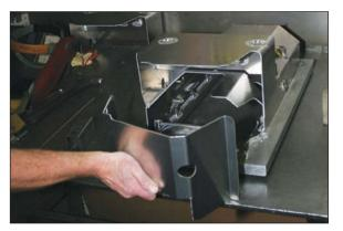
Moroso pioneered the deep and kick-out sump oil pan-here the deepest section of the pan begins to take shape. The efficiency of the CNC turret punch and bending processes ensure that each part is made to close tolerances, which means the actual welded seam is minimal in size.
