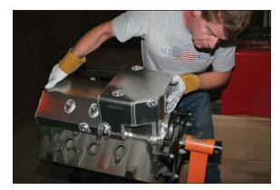
With all surfaces carefully welded, the completed pan is fitment checked on a real engine block. Moroso performs high-pressure leak tests on all fabricated Oil Pans.
