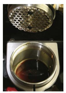
Volume of oil captured by Air-Oil Separator after 500 miles. (tested on 2010 Moroso Test Vehicle with 2,500 total mileage)
