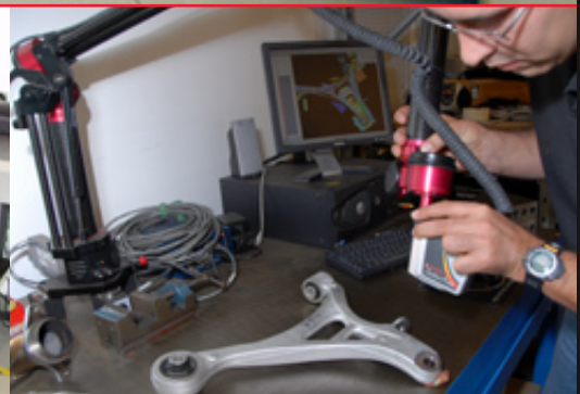
The 7-Axis Portable CMM equipped with laser scanner is also used to quickly and accurately inspect parts and surfaces.
