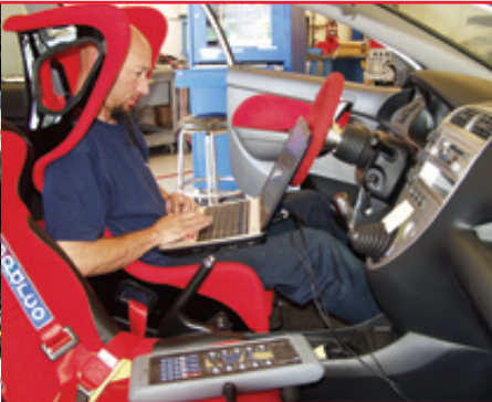
Dr. Charles seen here making final MAP adjustments to the Hondata ECU on the chassis dyno.
