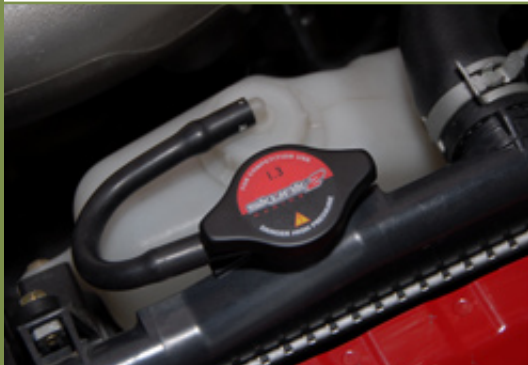
The Skunk2 radiator cap is a must for hard driving. It improves cooling by increasing the pressure inside the radiator.
