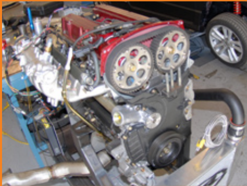
Mitsubishi EVO 4G63BT engine with Skunk2 Pro-Series cam gears mounted on an engine dyno test stand.
