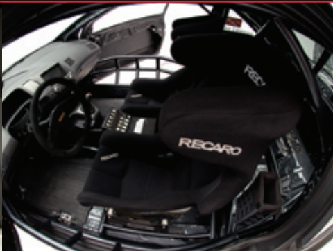
Interior view of the SiR2 with Braille/Recaro SPG seats and NASCAR style door bars for added protection.
