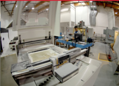
Large Format Z-Corp rapid prototyping machine. We are able to build color prototype 3D models as large as 20 x 24 x 16 using this machine.
