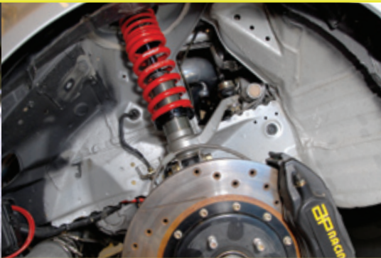
RSX-T front PRO-S suspension with included helper springs matched with AP Racing brakes. A potent combination.
