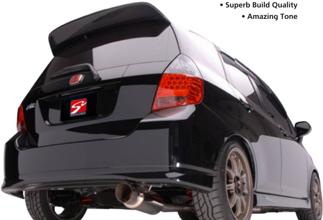
Unlike some manufacturers' silencers that are nothing more than horsepower restrictors, the Skunk2 silencer is engineered to be a free-flowing mini-muffler made from perforated stainless tubing wrapped stainless wool and mesh. This results in a significant reduction in noise with a minimal reduction in power when used.
