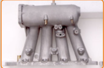
Clone: Looks similar to our first gen manifold. Clearly an inferior finish; rough and splotchy. We have noticed that clone manifolds are darker and more brittle (the fuel rail mounting bosses and corners of the head flange have a tendency to break off) this is usually an indication of inferior, usually recycled, aluminum being used.
