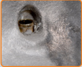
Clone: That black streaking is oxidation that results when the chemicals used to clean the manifold are not rinsed off properly. The large burr taken to properly finish and machine all areas of the manifold including areas you can't see. This burr is on the INSIDE of the manifold.
