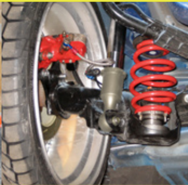
Pictured is the prototype PRO-C rear suspension used on the Fit R. Also notice the custom rear disc brakes.
