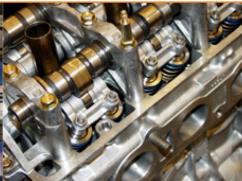
Yes, this is a picture of Beta's valvetrain. Skunk2 cams, valves, retainers, and Pro Valve Springs.
