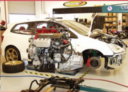
The RR's 2.4L 254whp K24 iVTEC engine getting lowered on to the front subframe.
