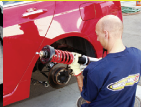
PRO-S rear suspension being installed onto the Skunk2 TSX. Dubbed as the M3 killer, this car outperformed the BMW M3 on the skid pad pulling 0.92g.
