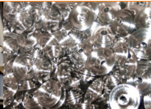
Great care is taken when machining our titanium retainers to ensure dimensional accuracy and a high quality surface finish free of stress risers.
