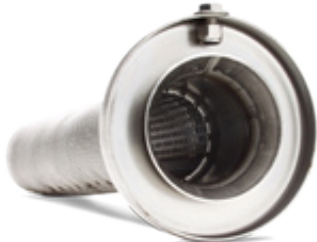
Unlike some manufacturers' silencers that are nothing more than horsepower restrictors, the Skunk2 silencer is engineered to be a free-flowing mini-muffler made from perforated stainless tubing wrapped stainless wool and mesh. This results in a significant reduction in noise with a minimal reduction in power when used.
