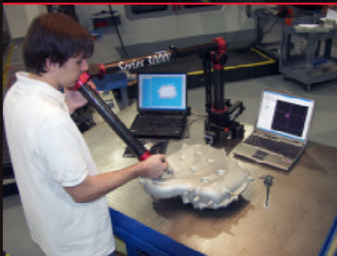
6-Axis CMM inspection arm allows us to accurately measure and inspect any object within +/- 0.001". That information is then imported into the CAD system and the parts are designed.
