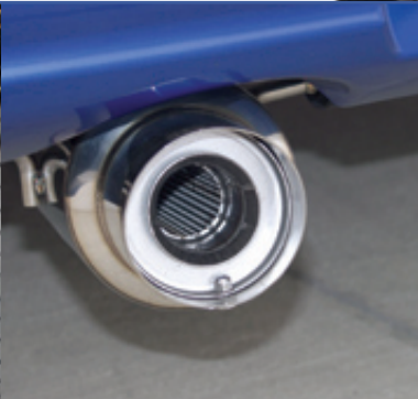
All Mega Power systems include removable silencers that are constructed as mini-mufflers.
