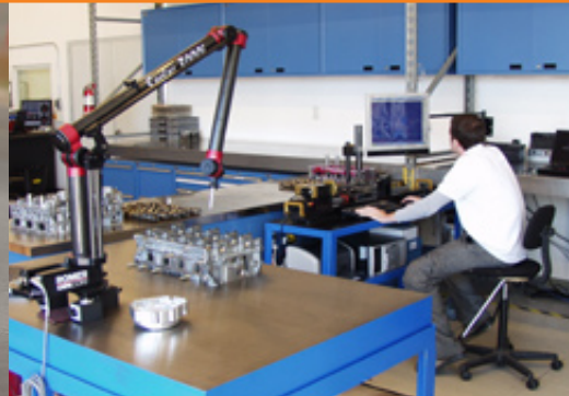
Before a cam can be designed, the cylinder head geometry must be measured and modelled in the CAD system.
