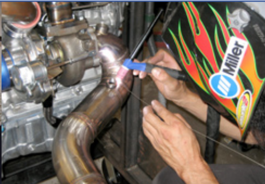
All exhaust component development starts out by hand fabricating and dyno testing prototype components.
