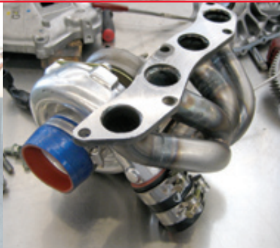
Honda requested that we use the stock 1.5L engine so we built a custom turbo kit for the FitR.
