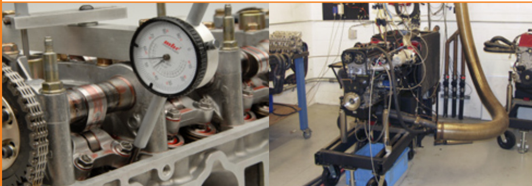
After the cam profiles are measured, we install the camshafts into engines to verify valve lift, valve timing, and lobe indexing.
