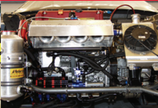
390 bhp 11,000 rpm engine with 5-stage dry sump oiling system.
