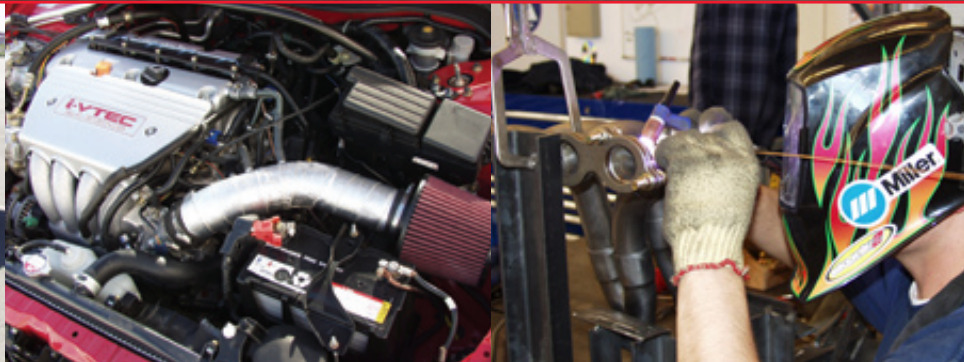
Skunk2 cams, header, exhaust, intake, and ECU program increased horsepower by 65whp.
