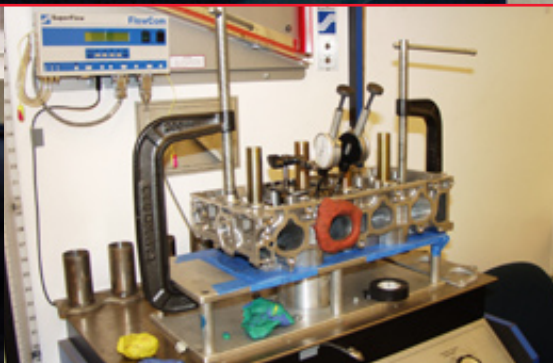
Equipped with computerized data acquisition our flowbench is used to measure the airflow through any part.
