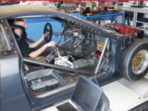
Fine tuning the Motec base map for Delta on the Superflow Chassis Dyno.
