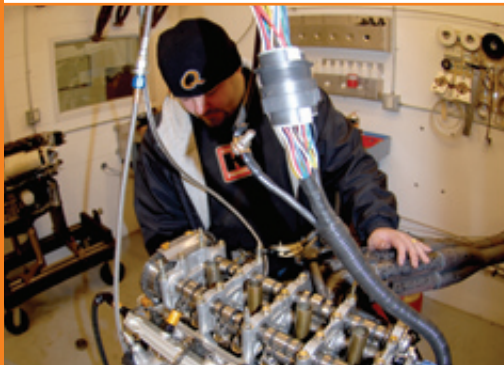
Skunk2 valvetrain components are performance and durability tested on the engine dyno. We'll hold the engine at various rpms for hours at a time.
