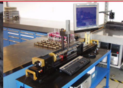
Camshaft measurement bench accurate to 0.00001" and one-hundredth of a degree. This machine is used to inspect and analyze camshafts.
