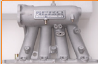
Skunk2: Each Skunk2 Pro-Series manifold features an acid etched stainless steel nameplate and superior consistent smooth finish. Skunk2 uses a high quality virgin 356 aluminum, which improves strength and finish. While marginally heavier, using a denser high quality aluminum makes the manifold significantly stronger.
