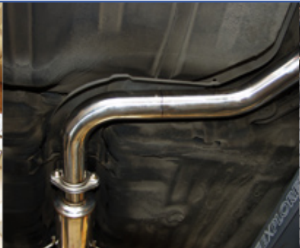
All Skunk2 exhausts are CNC mandrel bent, and carefully fitted to the car.
