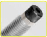
12-way adjustable valving dials in vehicle balance and feel.
