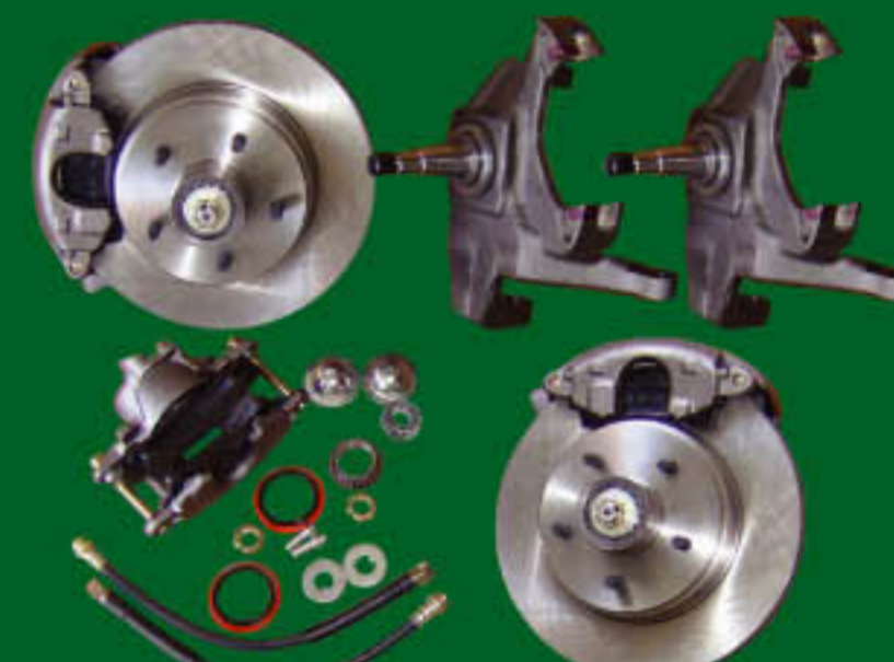
WBK2005 WYSCO 2" Drop Big Rotor 1967-1969 Camaro 2" Drop with Big 12" Rotors New 1 piece design spindle lowers car 2". Eliminates need for bolt on brackets. Steering arm "cast" one piece for precise factory geometry. Big brakes in an economical package. Requires 16" or larger wheels. Realign car after installation.
