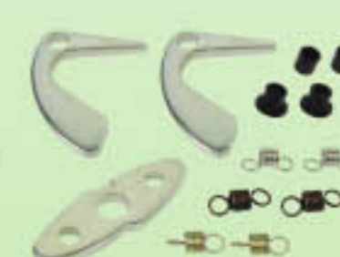
H. E. I. Advance Curve Kit Spring guide Copper=light Sliver=medium Brown=heavy WA9333 Chevy/GM V8
