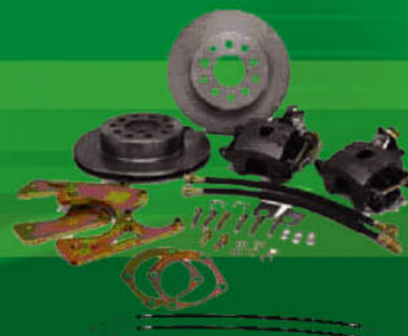
WBK2002 WYSCO 11" Rear Disc Brake Conversion Kit Fits 1965 and later Chevy 10 & 12 Bolt Rear ends. 11" Rotor with Cast Iron E-Brake (standard) Complete bolt on kit with E-Brake Cable. Maintains Factory rear Wheel width.
