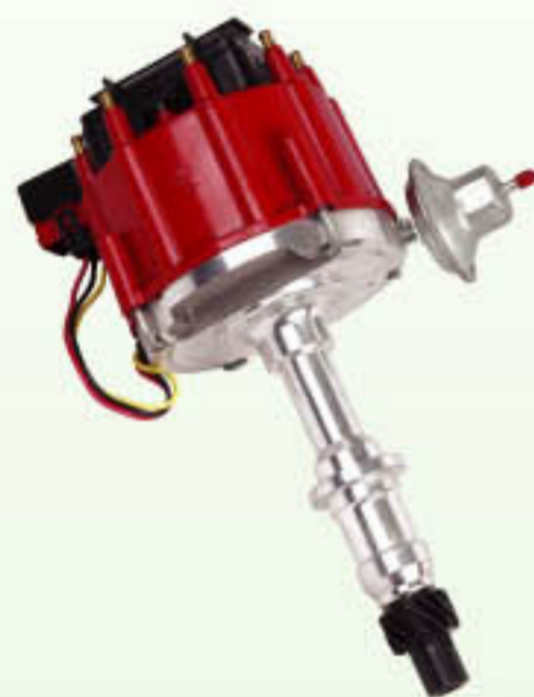
WP8912 Pontiac V8 350-455 HEI Distributor Red Cap 50,000 Volt adjustable Vacuum Advance
