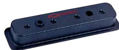
141-131.....Center hold-down, black crinkle, S/B with baffle
