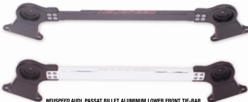
NEUSPEED AUDI, PASSAT BILLET ALUMINUM LOWER FRONT TIE-BAR Available in . . . ALL BLACK ANODIZED WITH RED FILLED NEUSPEED OR BLACK/POLISHED 45.10.60 / 45.10.60P
