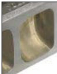
CNC-ported intakes are offered in both 345cc and 380cc sizes, with the exhaust ports also enlarged beyond the "as cast" 132cc port size. Heads are available bare or in complete assemblies.
