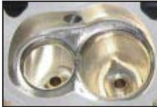
CNC-ported combustion chamber and bowls. Heads can be milled.
