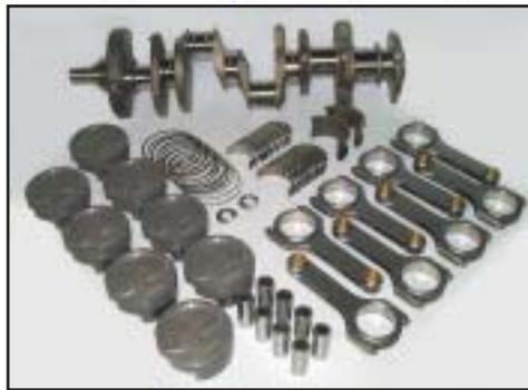
**SHORT BLOCK KIT AND ROTATING ASSEMBLY - Kit** contains a race-prepped Motown II iron block and an internally balanced rotating assembly with 4340 crank, H-beam rods, forged pistons, wrist pins, piston rings, plus rod and main bearings
