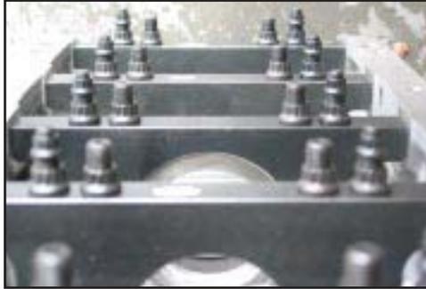
**The Warhawk' block is designed with priority main oiling so the bottom end gets fed first and "upstairs" last**
