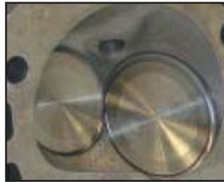
119cc combustion chamber with 2.300" intake and 1.880" exhaust
