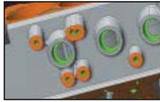
Motown II blocks are equipped with both front and side mounts for LS and standard SBC engine mounts.
