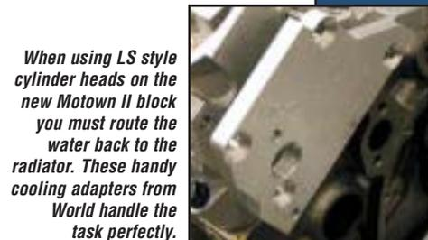
When using LS style cylinder heads on the new Motown II block you must route the water back to the radiator. These handy cooling adapters from World handle the task perfectly.
