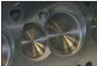
Highly efficient combustion chamber design plus larger diameter valves
