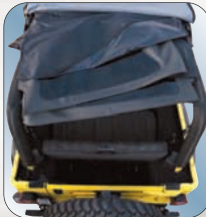
Open concealed ceiling storage panel Insert windows into protective storage pocket
