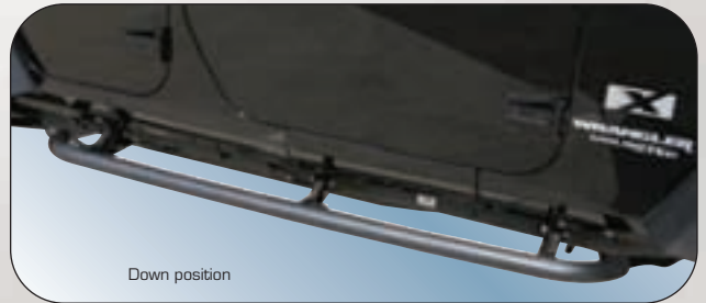
Dual purpose bar - step for street, rocker guard for offroad.
