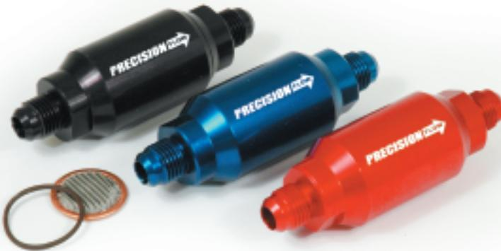
Replaceable disc style filter element allows for bi-directional filtering. Filter achieves flow rate of 95 Gallons/Hour at 7 PSI. Standard colors: Blue, Red, Black and Clear Anodize.
