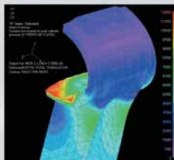
H-beam: Stress contour. Compression loaded at peak cylinder pressure of 1150 PSI@ 13°ATDC.
