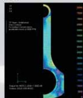
As in compression, this shows that the popular H-beam has some areas of high stress concentration at the beam to bore intersections.
