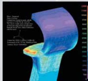
OLIVER: Stress contour. Compression loaded at peak cylinder pressure of 1150 PSI@ 13°ATDC.
