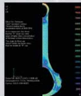
As in compression, this shows that the single rib OLIVER doesn't exhibit any higher stress than the popular H-beam.
