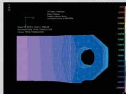
H-beam: Total transition contour. Loaded in tension due to acceleration force at 8000 RPM.
