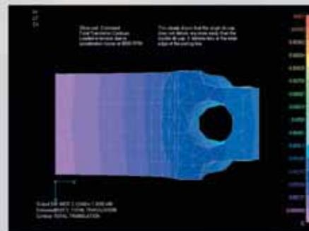
OLIVER: Total transition contour. Tension loaded due to acceleration force at 8000 RPM. It clearly shows the single rib cap deforms less than the double rib cap. It deforms less at the inner edge of the parting line.
