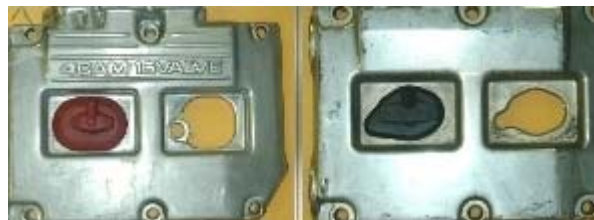
Oval shaped boot (hydraulic lifters) Teardrop shaped boot (solid lifters)
