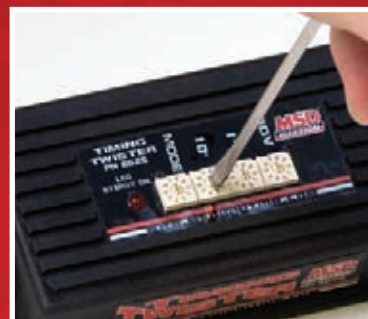
Adjustments to the timing are easily made with a twist of a rotary dial.
