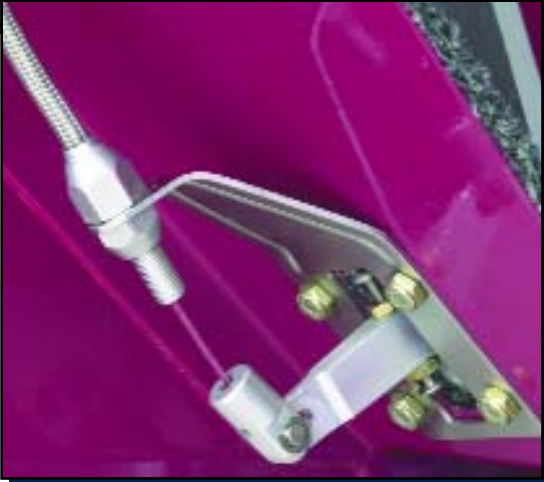
Under the floor cable mounting bracket
