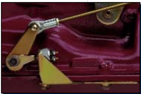
Single trigger shown for Back-Up Light
