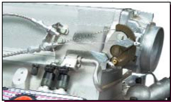
Use Ramjet Bracket with LS1 Throttle Cable
