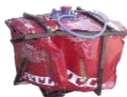
ATL Fuel Cell "Crash-Crunched" at 140 mph
