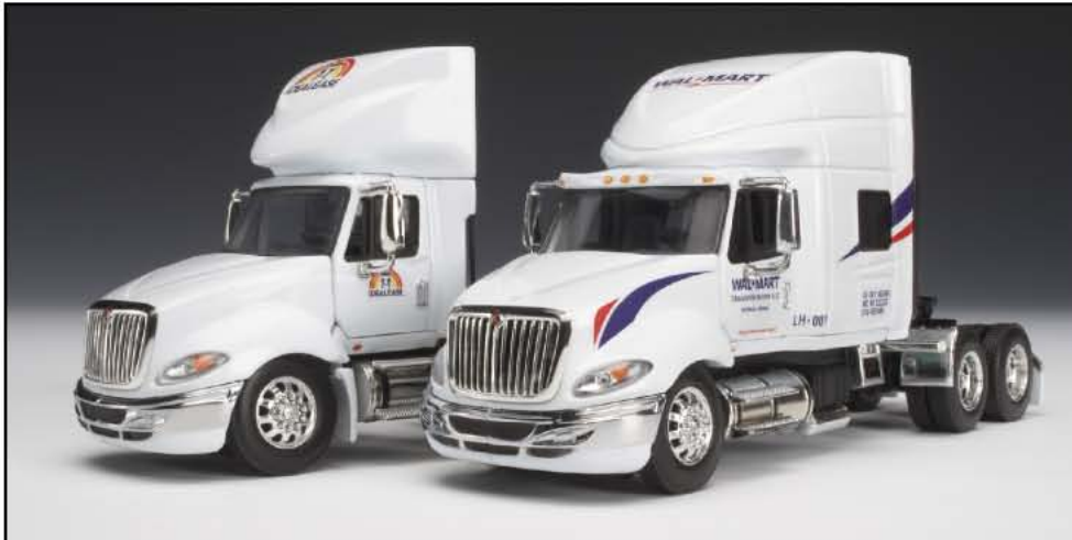
International ProStar Available with or without sleeper, with or without airfoil, with mid- or high-roof and with or without side skirts.
