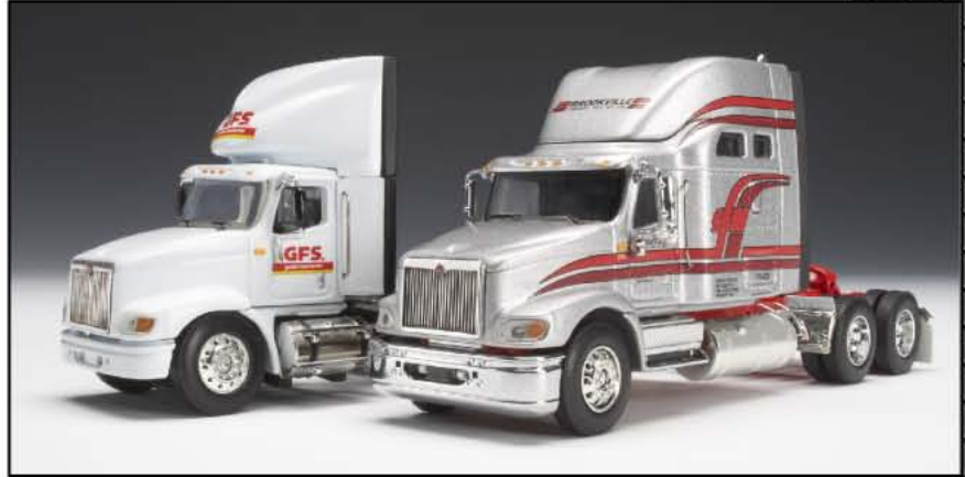
International 9100i & 9200i Available with or without sleeper, with or without airfoil, with mid-or high-roof and with or without side skirts. Day cab also available with or without Aeropod airfoil, cab extensions, and single or tandem axles.
