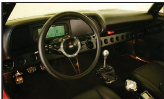
The UDX-SR Dash provides turn signals, high beam indicator, and even parking brake warning lights.
