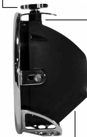
High Impact glass reinforced UV nylon housing to protect the integrated Gen 5 ballast & bulb
