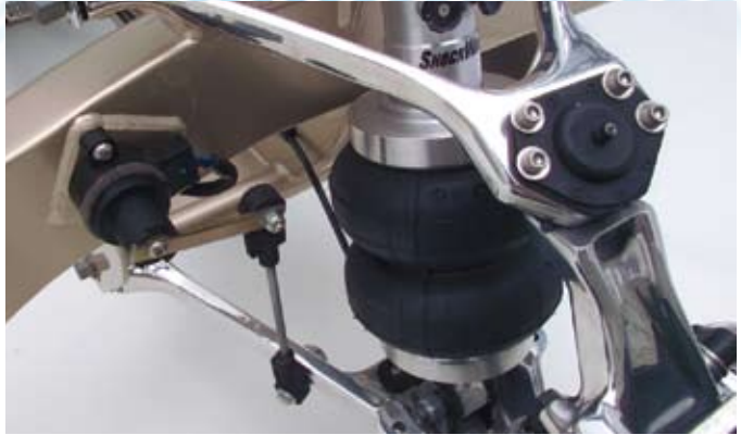
The ride height sensor is used to tell the computer the actual ride height of the vehicle.
