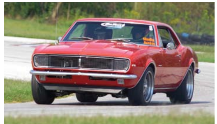
This 67 RS Camaro was set up with an AirBAR ® and ShockWaves ® in the rear and STRONGARMS ®, RideTech spindles, a MuscleBar ™ swaybar, and ShockWaves ® in the front. Notice on both the Chevelle and the Camaro how the outside tire now leans into the turn instead of leaning out like it does on an oem suspension.
