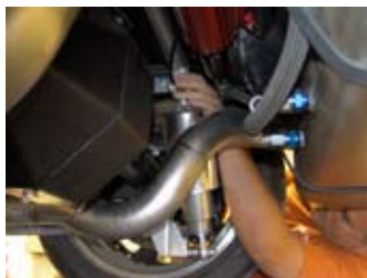
Run air lines to each air spring
