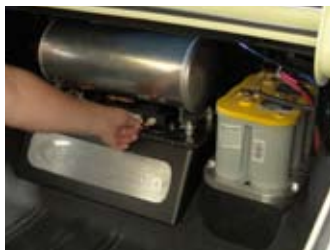
Run air lines to each air spring
