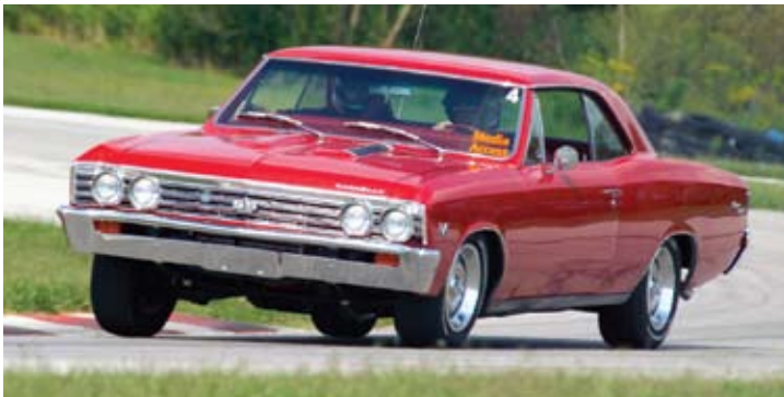
This 67 SS Chevelle is a restored original with stock suspension. Check out the body roll and how the outside tire leans out around the corner. This leads to poor lateral traction and unpredictable handling.
