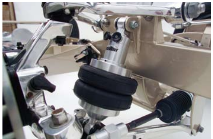
The ShockWave® is a patented combination of an air spring and a shock absorber. In this application it is a bolt-in replacement for a coilover shock.
