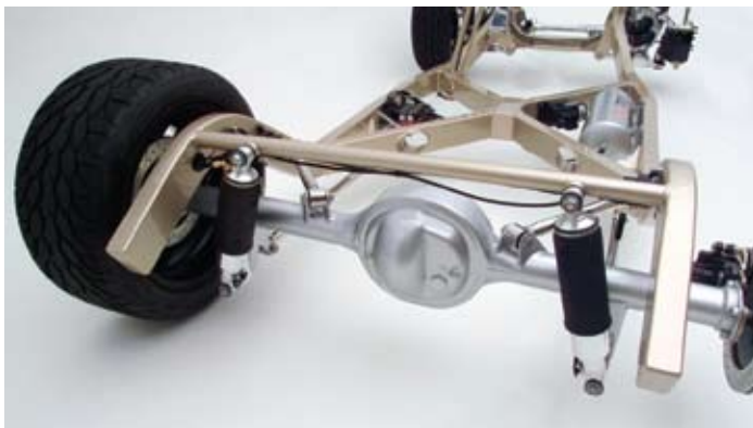
The 7000 series ShockWave® is a replacement for a conventional coilover on a 4 link or ladder bar style rear suspension. It has more travel and less spring rate than the double convoluted style ShockWave® that is typically used for a front application.
