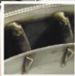
Tig welded turbine hub and furnace brazed fins
