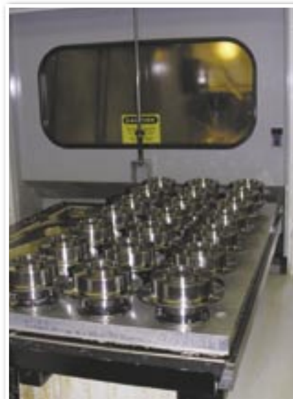
CNC machining of hubs and inner shells at the ATI facility
