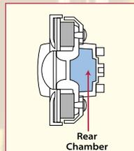
The rear chamber provides greatly improved damping and an extended midrange frequency response.
