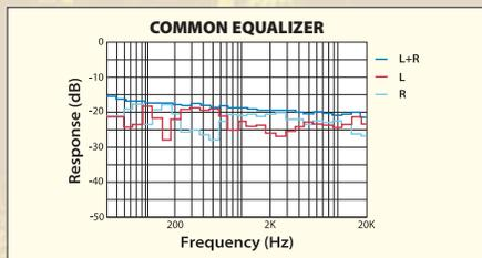
With an L/R common equalizer, the frequency response is a blend of the responses of the L and the R channels which have peaks and dips caused by the difference in acoustic characteristics. This non-flat response of the L and the R channels makes it difficult to create natural sound staging and imaging.
