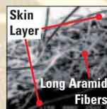
Aramid Fiber Reinforced IMPP Cone
