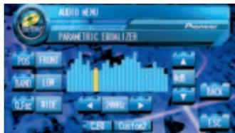
Screen for controlling the parametric equalizer.
