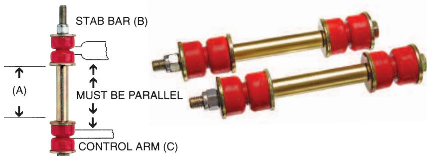
**TO FIT:** Vehicle must be on level ground (not jacked up) with wheels supporting it. Make sure stabilizer bar end eyelet (B) is parallel with control arm (C). Many times they are not. You may be required to use a slightly longer or shorter sleeve length than the original. Measure sleeve length.
