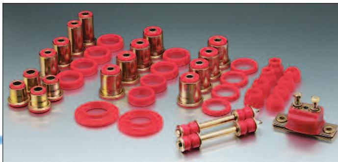
Unfortunately, large, soft O.E.M. rubber bushings cause sway bars, shocks, control arms etc., to deflect and cause inconsistent
