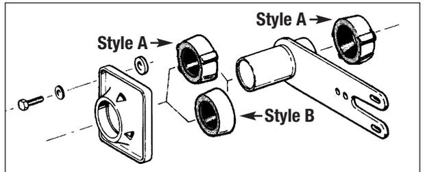
Due to the many variations of suspensions on Baja bugs, sand rails, etc., these Rear Spring Plate Bushings are sold two ways.
