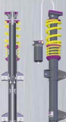
The upside down McPherson struts design, where the damper cartridge is placed inverted in an outside tube, absorbs optimal the site forces by the outside tube. The plain bearing or the linear bearing which are placed in the outside tube assures a less friction of the damper at work. That is the reason why the dampers have a fast responding and a less breakaway torque.
