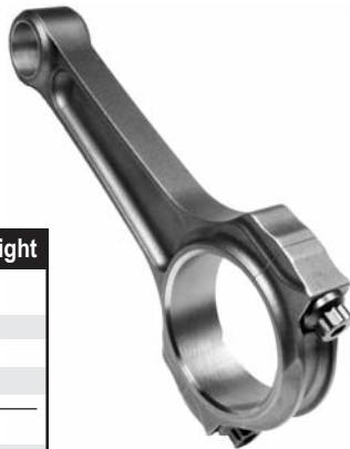
All Dirt Series connecting rods are supplied with 7/16" ARP 2000 cap screw fasteners P/N 42390. Upgraded 7/16" ARP Custom Age 625+ cap screws P/N 42252 are available. To order upgraded fasteners, affix an "R6" after the rod part number.
