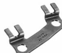
To convert Ford 351C engines to adjustable rocker arms and pushrod guide plates, machine the old rocker stanchions down to a height of .550" as measured from the adjacent head bolt spot face with cutter 41860. Drill and tap the old screw hole to accept stud 42277.
