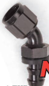
Lightweight synthetic rubber inner-supported by a extruded elastomer outer jacket, uses push to assemble barb technology for simple assembly rated to 250 PSI.
