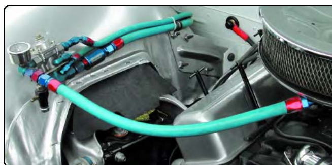
Lightweight synthetic rubber inner-supported by a extruded elastomer outer jacket, uses push to assemble barb technology for simple assembly rated to 250 PSI.
